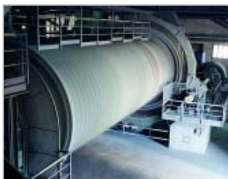
Examples of cement mills seated on trunnion bearings.
